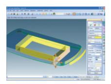
With the explicit approach, you can make instant design changes through on-the-fly interactions with model geometry.
