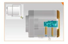
You can use the Move by Box command to enlarge an electronic enclosure to accommodate a new, larger circuit board, for example.
